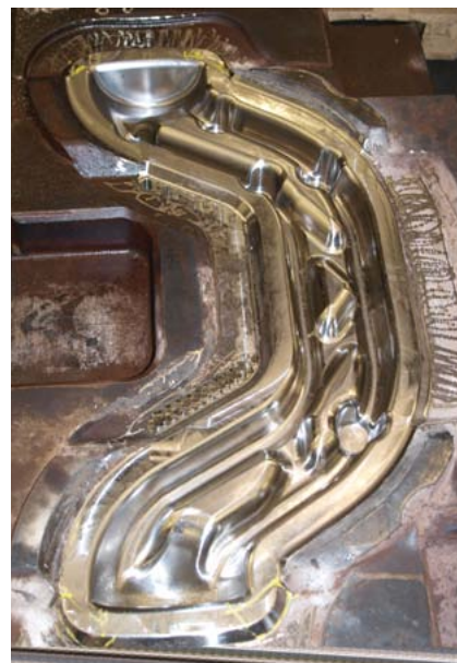
Fully welded die after machining
